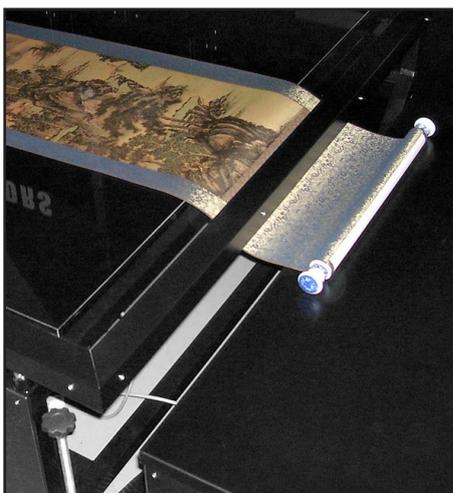
The distance between the glass and the table surface can be easily adjusted between 0 to 15cm in order to accept originals up to 15cm thick or work without any contact with the glass (focus will be done under the glass).
